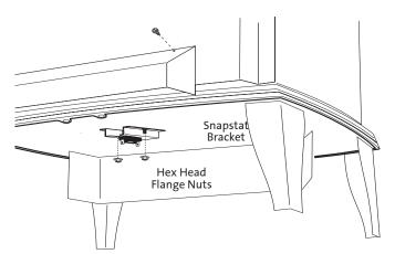
Figure 34. Attach Snapstat Bracket.
